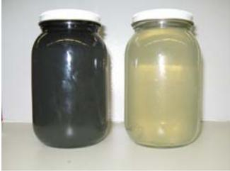
Figure 3. Dirty and clean cooling water samples
